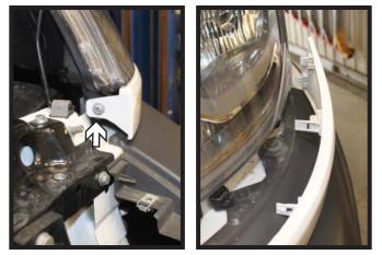
3. Using a phillips screwdriver, remove the screw from the fascia panel under the headlight. Unsnap the panel and set aside. Do this on both sides of the vehicle.
