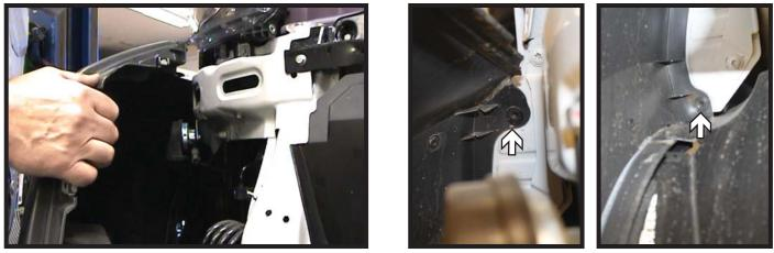
7. Pull the corner of the fascia away from the vehicle, using a 30 Torx, remove the two (2) screws from the behind of the fascia. Do this on both sides of the vehicle. Disconnect any electrical lines and set the fascia aside.
