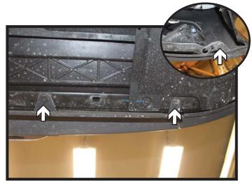
Using a T30 Torx, remove the six (6) screws from the underside of the fascia. There are three (3) on each side.
