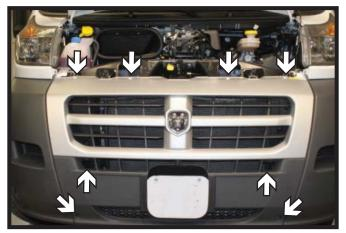
1. Using a T30 Torx, remove the eight (8) screws from the grille. Remove the grille and set aside.
