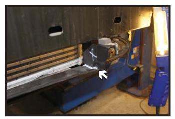
9. Trim off the lower shielding as shown and remove from the vehicle. Do this on both sides of the vehicle.
