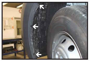
4. Using a 8MM socket, remove the three (3) screws from the wheel well. Do this on both sides of the vehicle.
