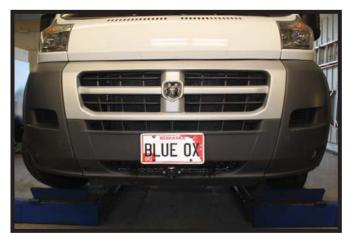
16. Hold the fascia as close to its original position, mark and trim the fascia around the convenience links and attachment tabs. Reinstall the fascia support, fascia panels, fascia and grille.
