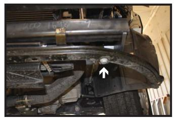
11. Using a 13MM socket, remove the bolt from the driver side fascia reinforcement.
