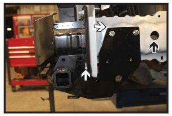
13. Using a 1-1/4" hole saw, enlarge the existing hole in the frame (black). Do this on both sides of the vehicle.
